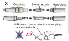
Fit the enclosed blower nozzle to the coupling and attach to the handpiece. Run idle with no water for at least 5 sec to clear
