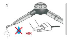
After removing the cleaning powder in the powder case, perform idle running with air alone to discharge water and powder in the nozzle.
