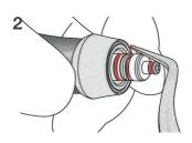
If powder adheres to the O-ring section, remove the O-rings, and carefully clean the O-rings and grooves.
