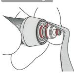
Replace the O-ring(s) at the handpiece joint section of the powder case, apply a drop of the enclosed turbine oil and rub it in with your fingers.
