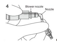
Use the blower nozzle in the same way to clear the lines in the Prophy-Mate neo nozzle. Blow from the far end of the nozzle.
