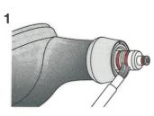
Carefully clean the inside of the joint section of the handpiece and the O ring section of the powder case with the attached cleaning brush.
